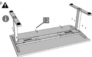
Attached the Control Box (part 6) to the underside of the desktop with two (2) M5x16 Wood Screws (part 14) close enough to one Leg (part 1) so that the cable from the Leg (part 1) reaches the Control Box (part 6). Connect the cable on the Leg (part 1) closest to the Control Box (part 6).
