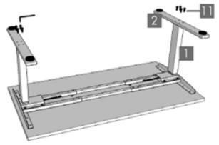
Double-check that the wood screws are not too long for your desktop and won't puncture the surface when screwed all the way in.
