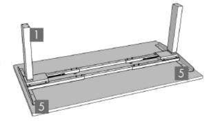
Using the supplied Allen Wrench and eight (8) M6x14 CS Machine Screws (part 12) attach the Lifting Columns (part 1) to the Frame Ends (parts 3a and 3b)
