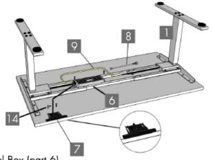
Connect the Cable (part 9) to the other Leg (part 1) and to the Control Box (part 6).
