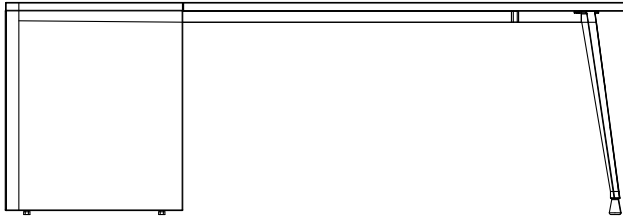
Standard Run-Off Connection (Desk Shell with Run-Off) 24" Depth Desk Shell with Flushed Modesty Shown
