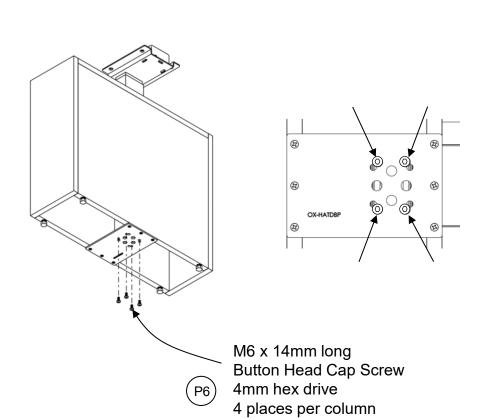
**Step 4:** Install feet. (only for columns without storage or stand-alone leg) If Columns require a storage piece or glide, skip this step and proceed to Step 5.
