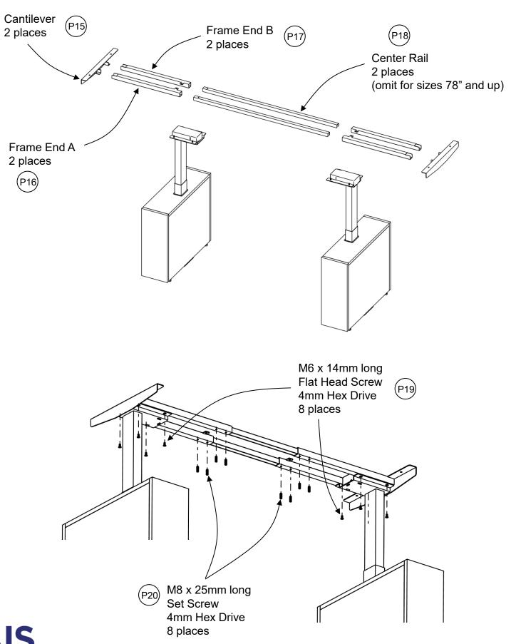
**Step 9 (for 3 leg configurations)**: Install the worksurface support components to the height adjustable columns for the return leg.
