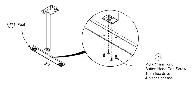
**Step 5:** Install Glide and Glide Plate (only for columns without storage or feet) If Columns require a storage piece or foot, skip this step and proceed to Step 6.
