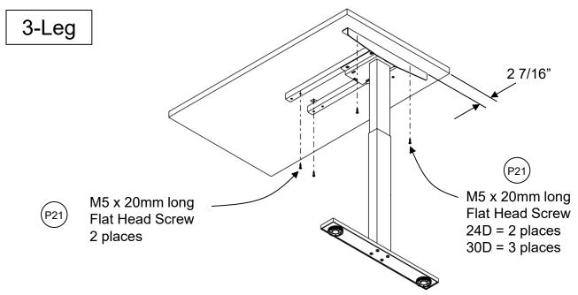
Step 13 (for 3 leg configurations): Align the return worksurface to the main worksurface. Secure in place using (2) U-Channels and #9 x 7/8" screws.
