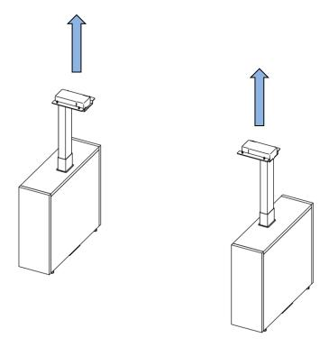
Step 8: Install the worksurface support components to the height adjustable columns.
