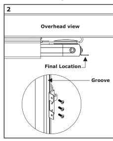
**Step 3 -** Install Cam and Core Cylinder on Lock Cover.
