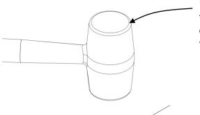
Use a non-marring mallet to GENTLY tap hinge down until flush with the top of the hanger rail.
