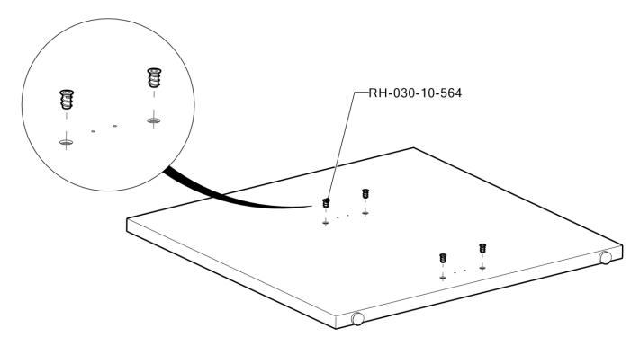
Install End Panel Braces with work surface screws, use the pilot holes provided.
