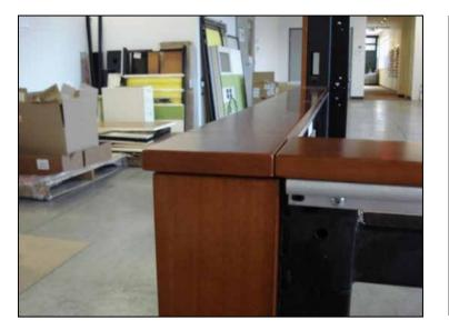
View of topcap assembly from side. Not that topcaps EXTEND out over connector cover. This is the proper position. Vertical covers are designed to align with tile faces.
