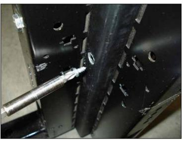
For bottom of connector locate pre-drilled relief holes on "inside" corner of connector body. Holes are ½ inch holes. Insert Screw A on extended #2 Phillips "shank" or hand screwdriver though hole and then through hole on the far side of connector as shown below...Tilting the vertical cover slightly to see screw emerge is acceptable.
