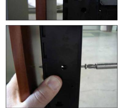
Insert LONG SCREW, Screw B, into standard connection hole approx 8 inches down from top of frame, immediately below top electrical chase cutout. This may require removal of sheetmetal captured nut from inside of frame. Align tip of screw with predrilled hole in endcap and attach endcap...
