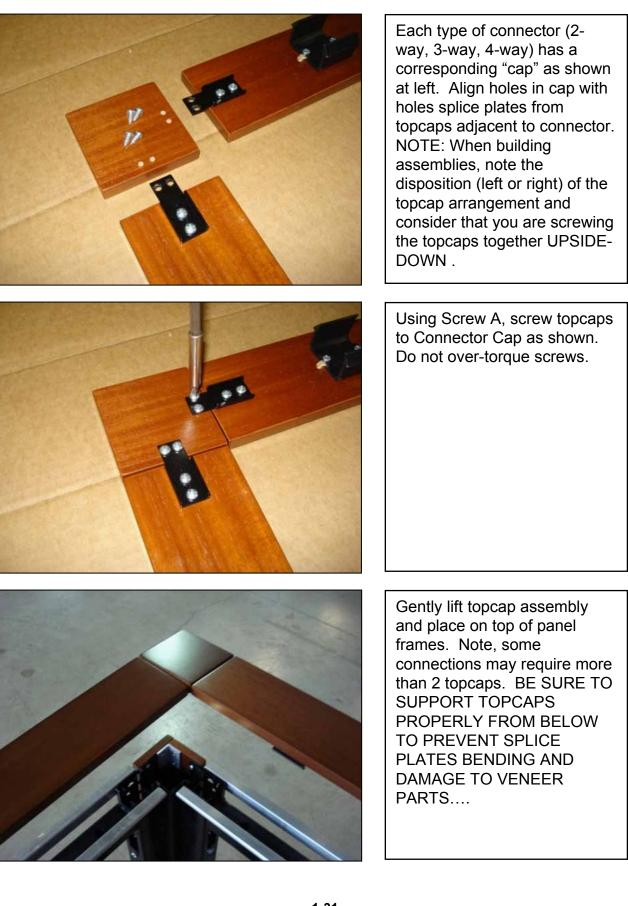
With topcap assembly resting on top tile retainers, apply pressure above clips to "snap" topcaps on to frames as shown.
