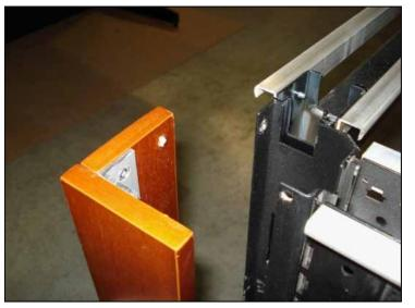
Install top tile retainers per standard Matrix install instructions. NOTE TRIM MUST BE INSTALLED WITH TILES REMOVED. In most cases, connector covers will be preinstalled at factory. However, covers may need to be removed for data routing. Simply line up the predrilled holes at the top of the connector body with the holes in the top of the cover....
