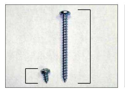
Matrix veneer trim installation uses 2 screw lengths. **FAILURE TO USE EXACT SCREWS PROVIDED** will damage the veneer product. Short Screw (A) = #8 Pan Head Sheet Metal Screw, #2 Phillips Drive, ½ inch long from TOP of head to tip. Long Screw (B) = #10 Pan Head Sheet Metal Screw, #2 Phillips Drive, 2 3/8 inch long from TOP of head to tip.
